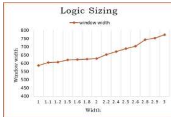
Fig 8: Graph showing variation of window width with transistor width.
