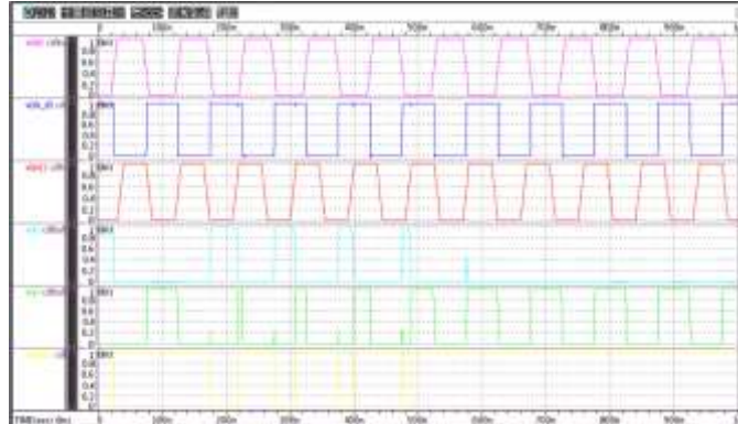
Fig 11: Wave view of buffer using Constant Delay Logic
